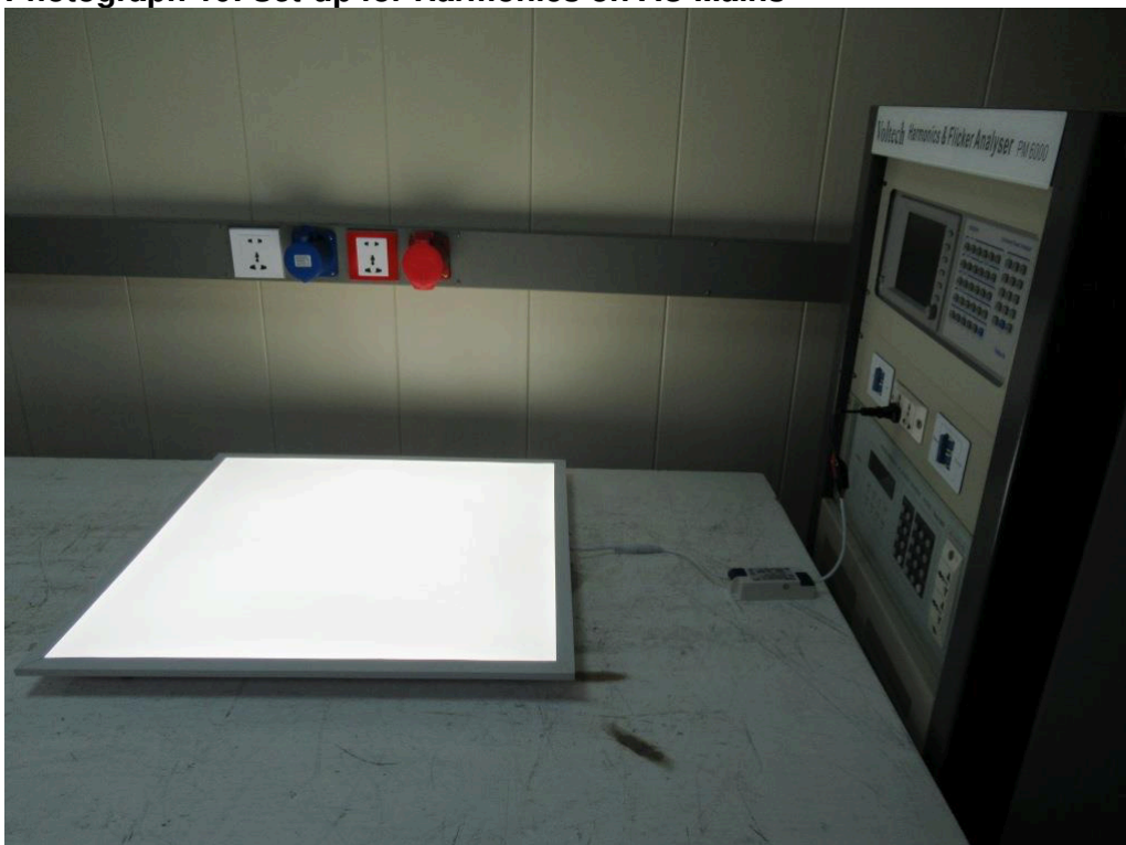
Photograph 10: Set-up for Harmonics on AC Mains
