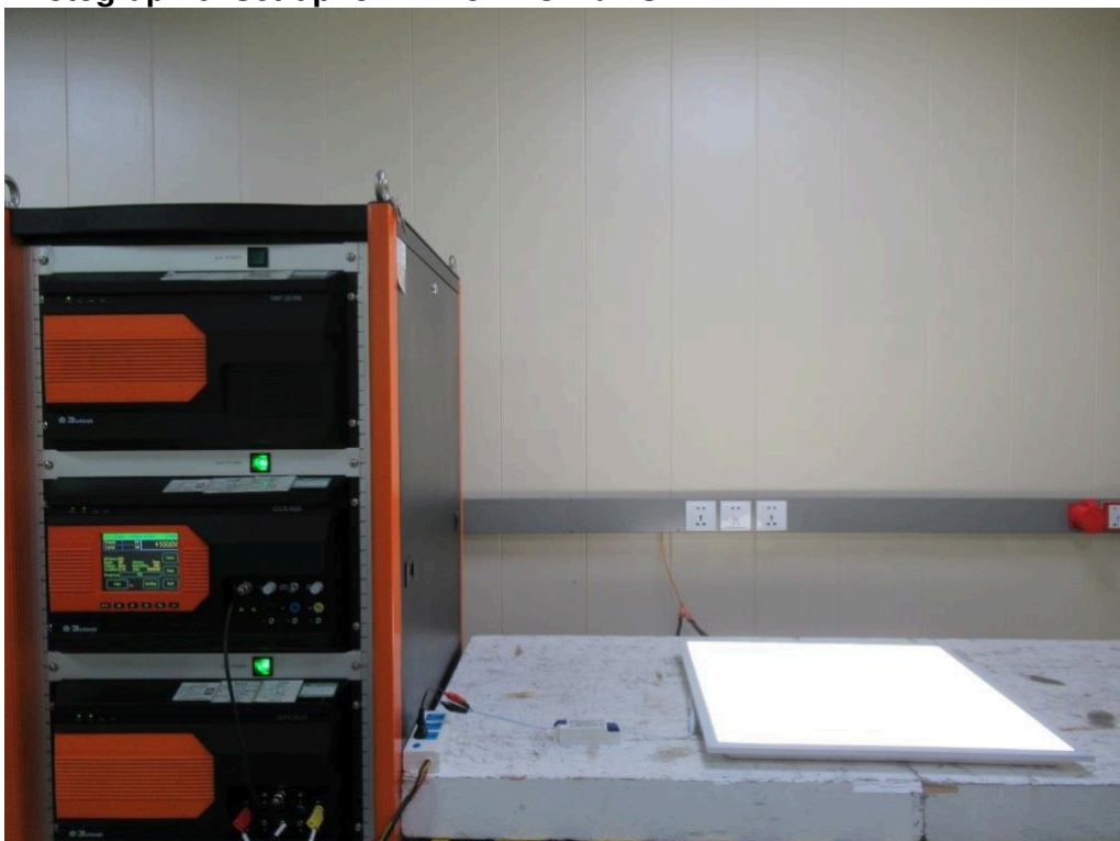
Photograph 6: Set-up for EFT on AC Mains
