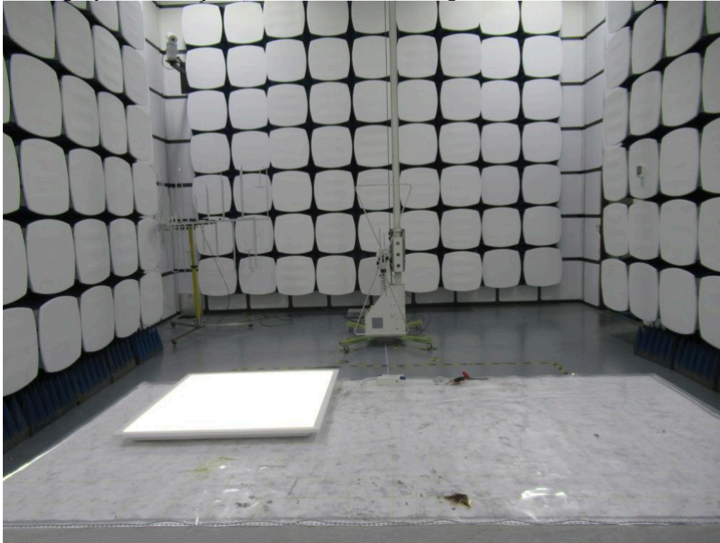
Photograph 4: Set-up for Radio Frequency Electromagnetic Fields (RS)
