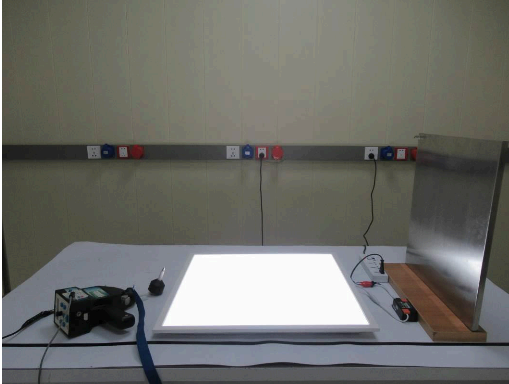
Photograph 10: Set-up for Harmonics on AC Mains
