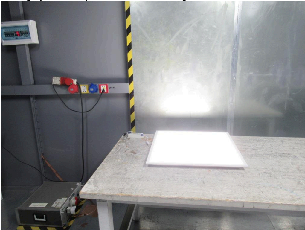
Photograph 2: Set-up for Radiated Electromagnetic Disturbances (Table 3a)
