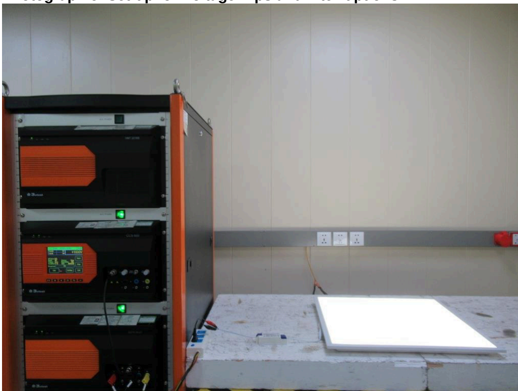
Photograph 8: Set-up for Voltage Dips and Interruptions
