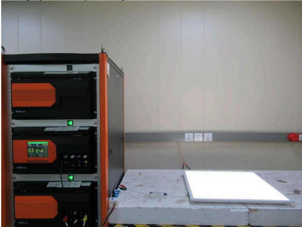
Photograph 8: Set-up for Voltage Dips and Interruptions
