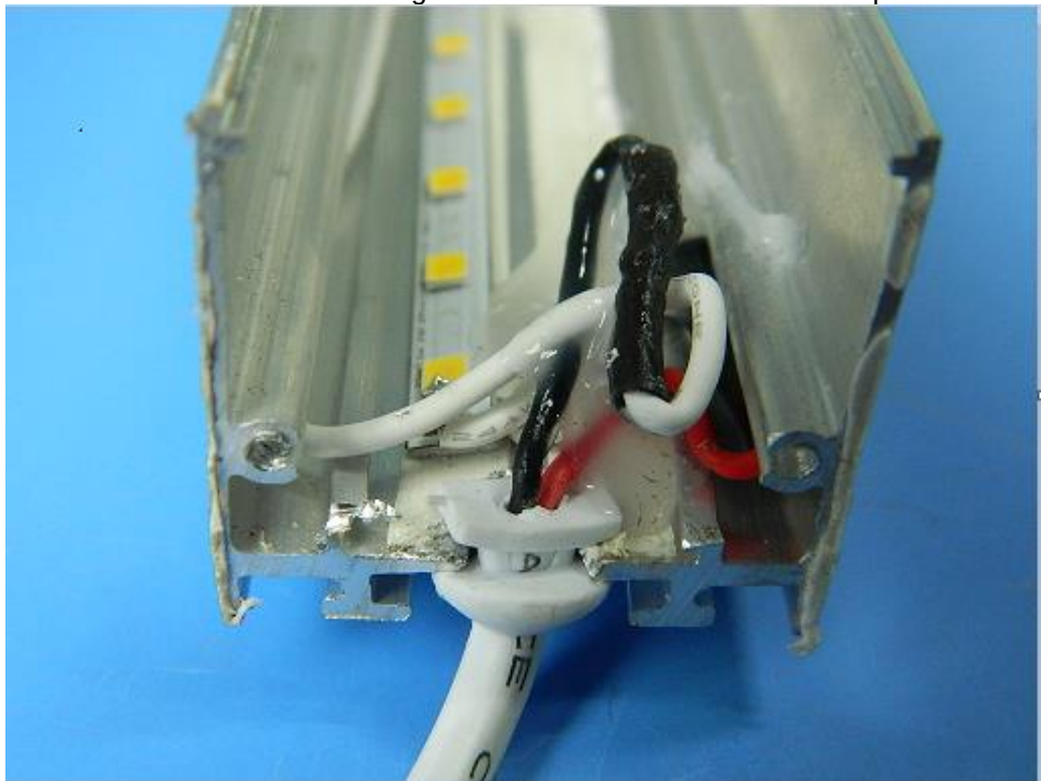
Figure 27: the inside view of TLPL-A-300-CW-2835
