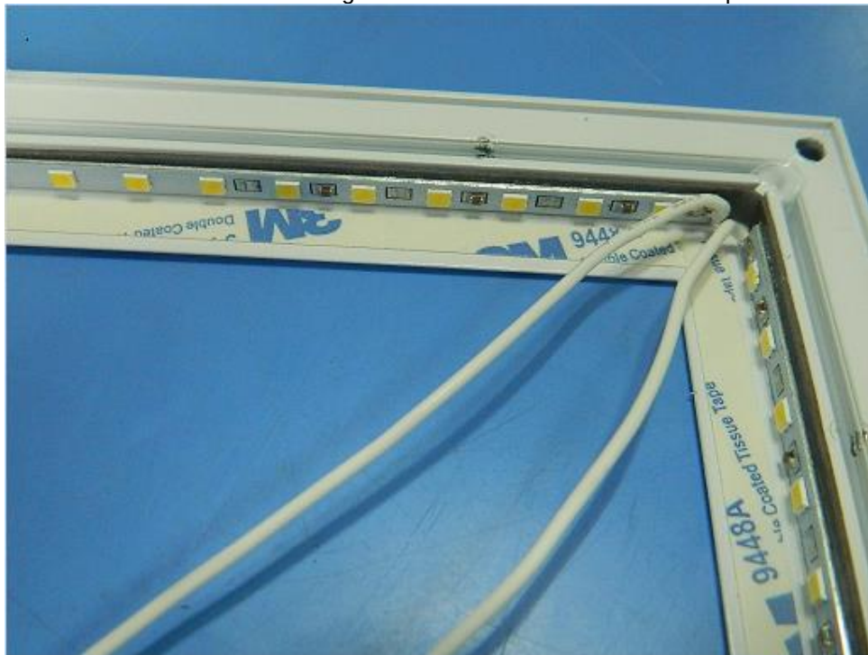
Figure 11: part of LED module
