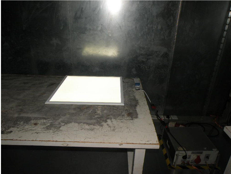
Photograph 2: Set-up for Radiated Electromagnetic Disturbances (Table 3a)
