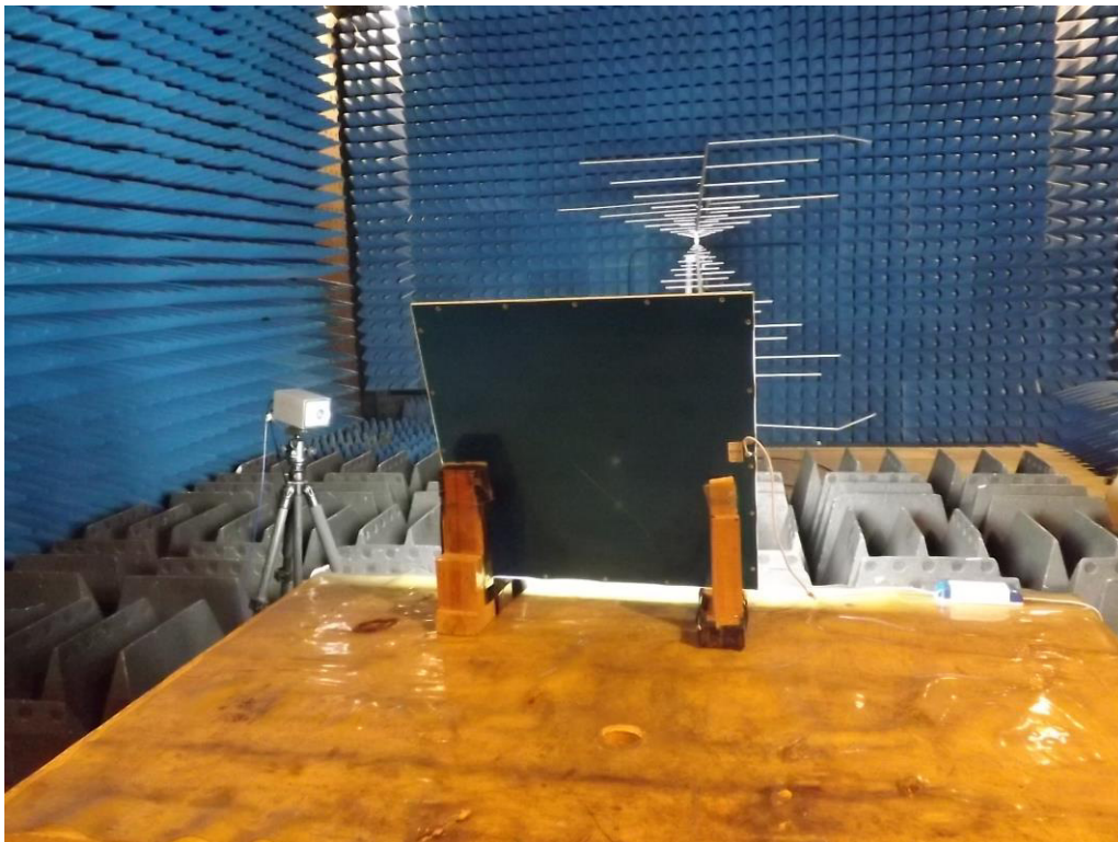
Photograph 4: Set-up for Radio- Frequency Electromagnetic Fields Susceptibility
