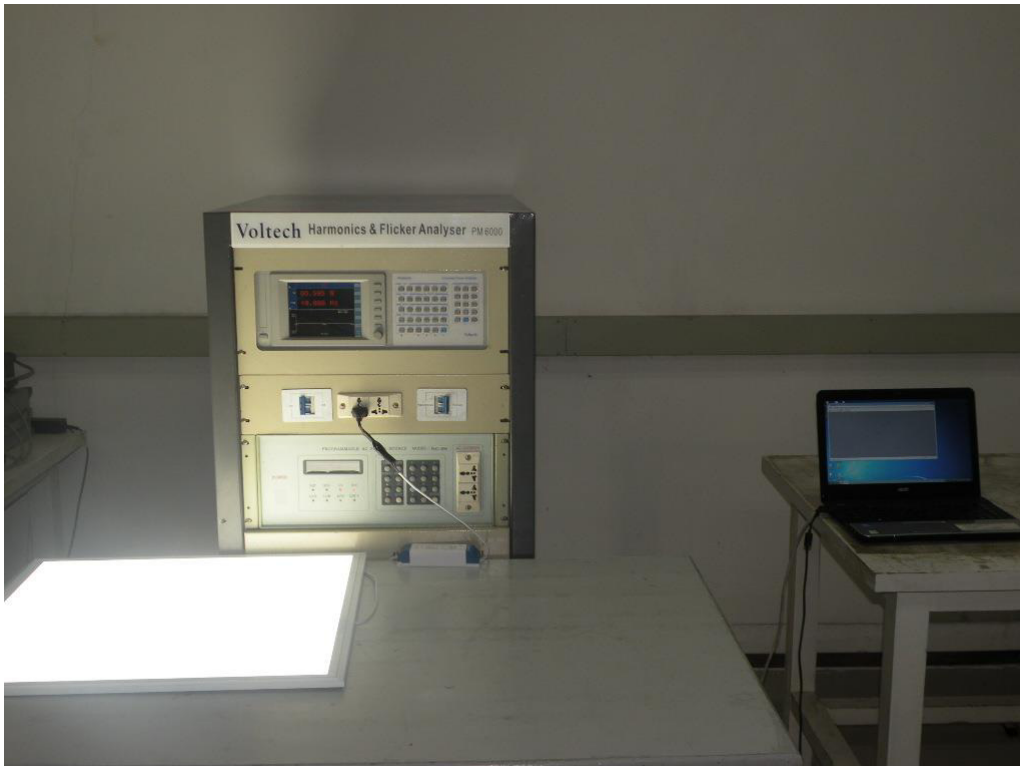
Photograph 10: Set-up for Harmonics
