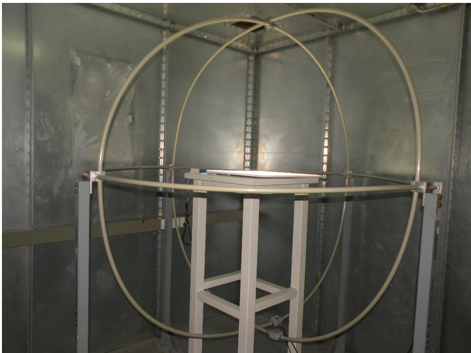
Photograph 2: Set-up for Radiated Electromagnetic Disturbances (Table 3a)
