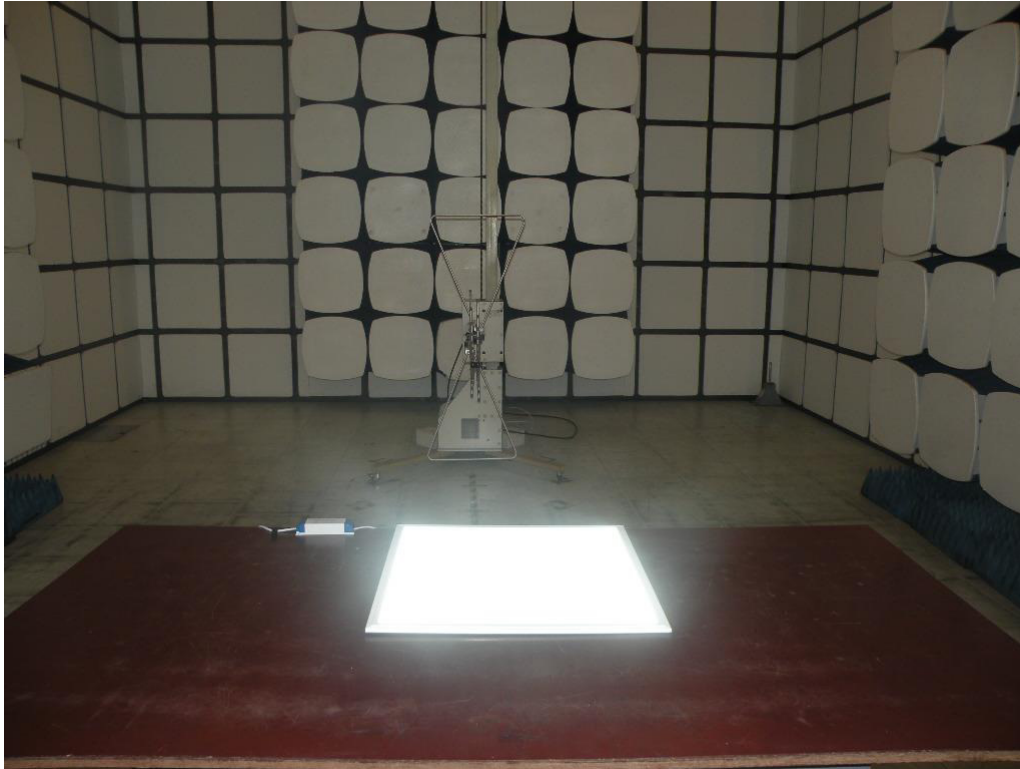
Photograph 3: Set-up for Radiated Electromagnetic Disturbance (Table 3b)
