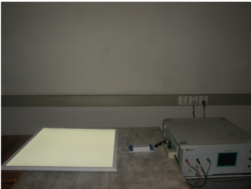
Photograph 6: Set-up for EFT
