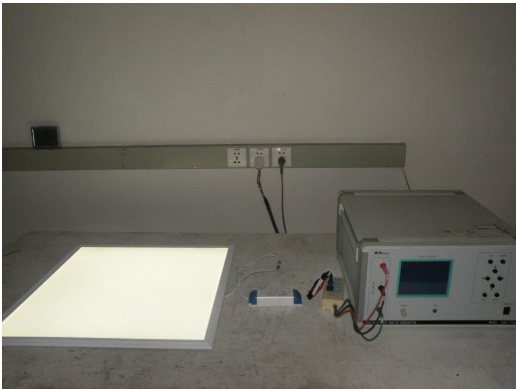
Photograph 8: Set-up for Voltage Dips
