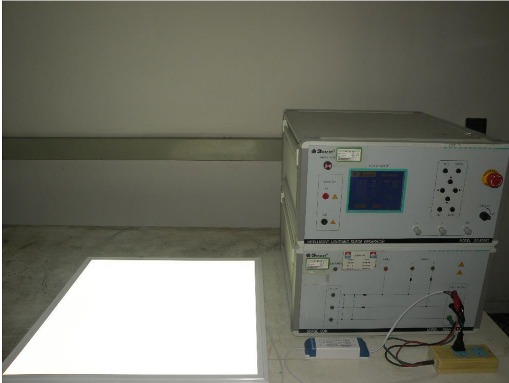
Photograph 7: Set-up for Surge
