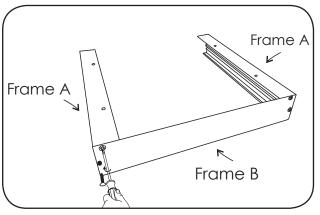
2 Fix the two 'A' frames together with one 'B' frame.
