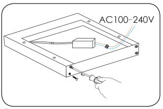
**6** Fix the 'B' frame with the screws supplied.
