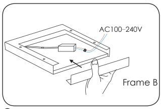
**5** Insert the other 'B' frame on to the ends of the 'A' frames.
