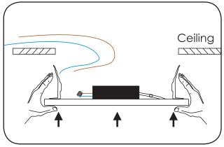
4 Connect the LED Driver to AC mains power. Push the LED Panel into the ceiling cavity with the springs raised.
