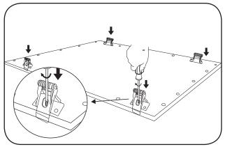
2 Place the springs in position and reinstall the four screws. (the screws must be inserted through the center hole of the clip as illustrated above).
