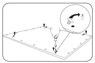
1 Unscrew the highlighted screws from the four corners of the LED Panel.
