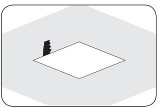
3 Cut a square hole in the ceiling 10mm smaller than the LED Panel.
