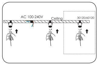
6 Screw the suspended cable to the ceiling fixture.
