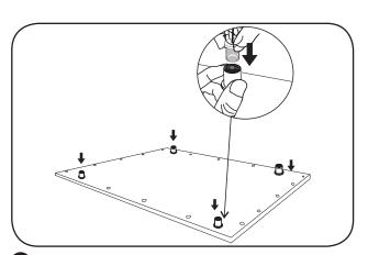
4 Screw the suspended cable to the LED Panel.
