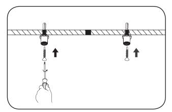
1 Insert the wall plugs into the ceiling and secure the suspended surface fixture to the ceiling.
