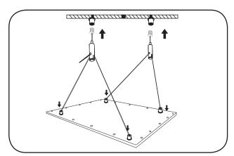
8 Fix the LED Panel to the ceiling and make final adjustments for desired height and angle.
