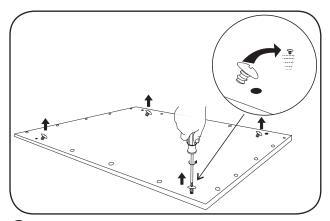
2 Unscrew the highlighted screws from the four corners of the LED Panel.
