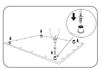
**3** Screw the suspended panel fixture to the LED Panel.
