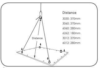
**5** Adjust the length of the suspended cable to the desired length.
