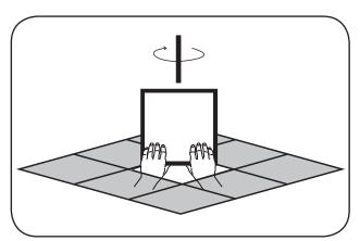
**5** Rotate the LED Panel to insert easily in to the ceiling grid.
