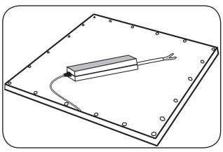
2 Place the driver on the back of the LED Panel.
