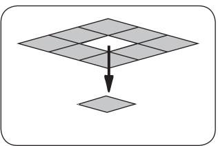
3 Remove the ceiling grid panel.
