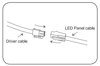
1 Connect the LED Panel cable to the DC side of the LED Driver.
