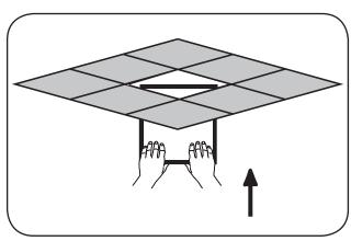
4 Insert the LED Panel into the ceiling grid.
